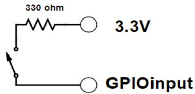
Graphical wiring of internal Resistor pulling the GPIO 14 pin high\*
