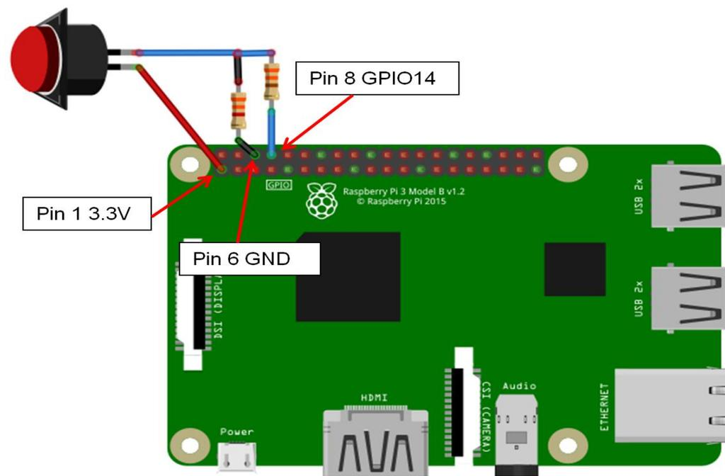
Schematic of external Resistor pulling the GPIO pin low
