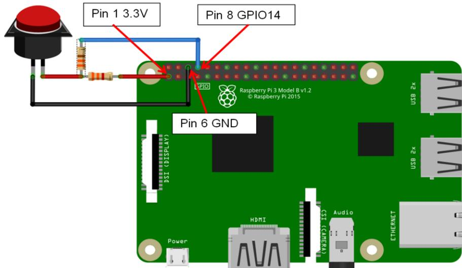
Schematic of external Resistor pulling the GPIO pin high
