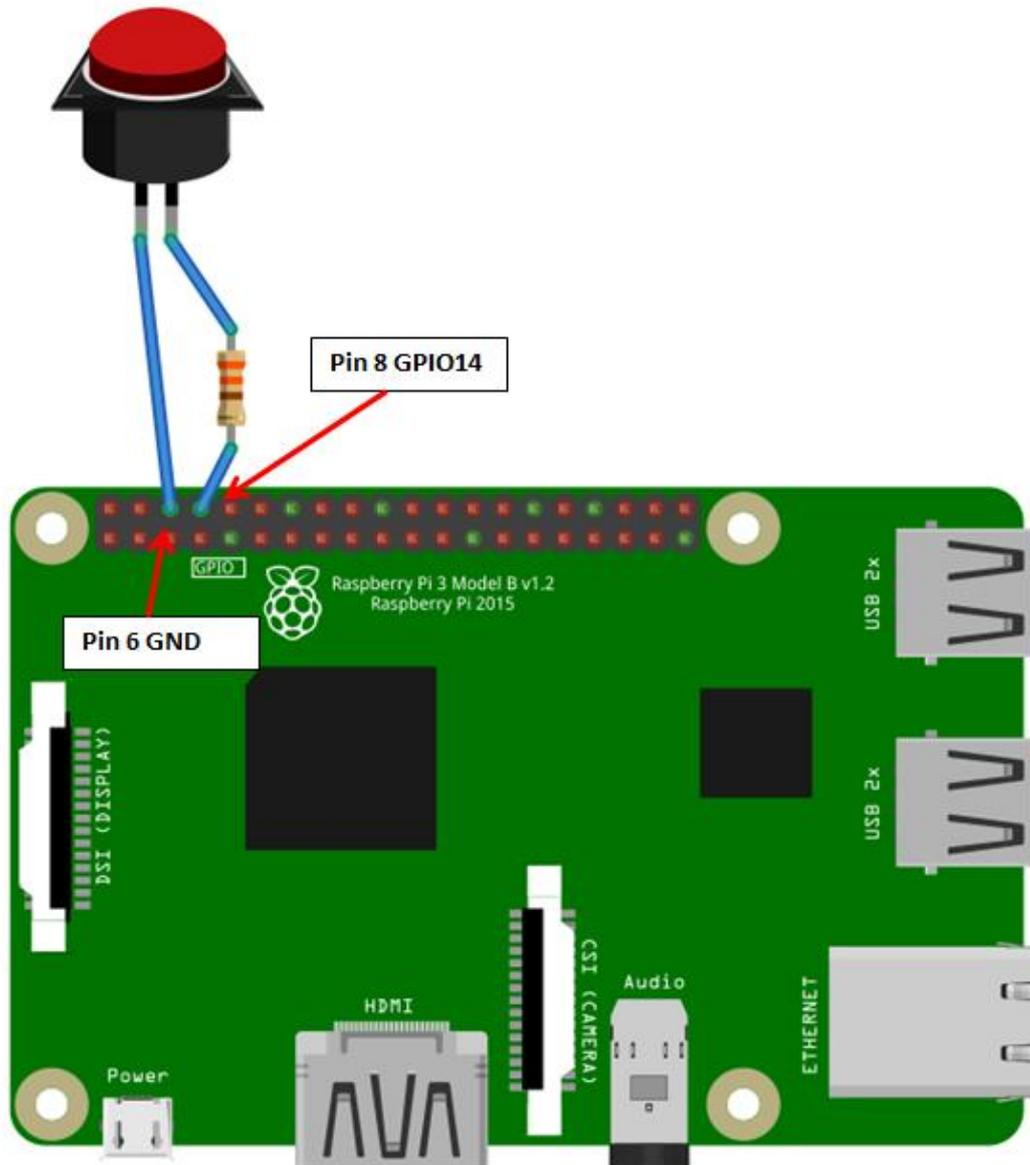
Schematic of Internal Resistor pulling the GPIO pin high\*
