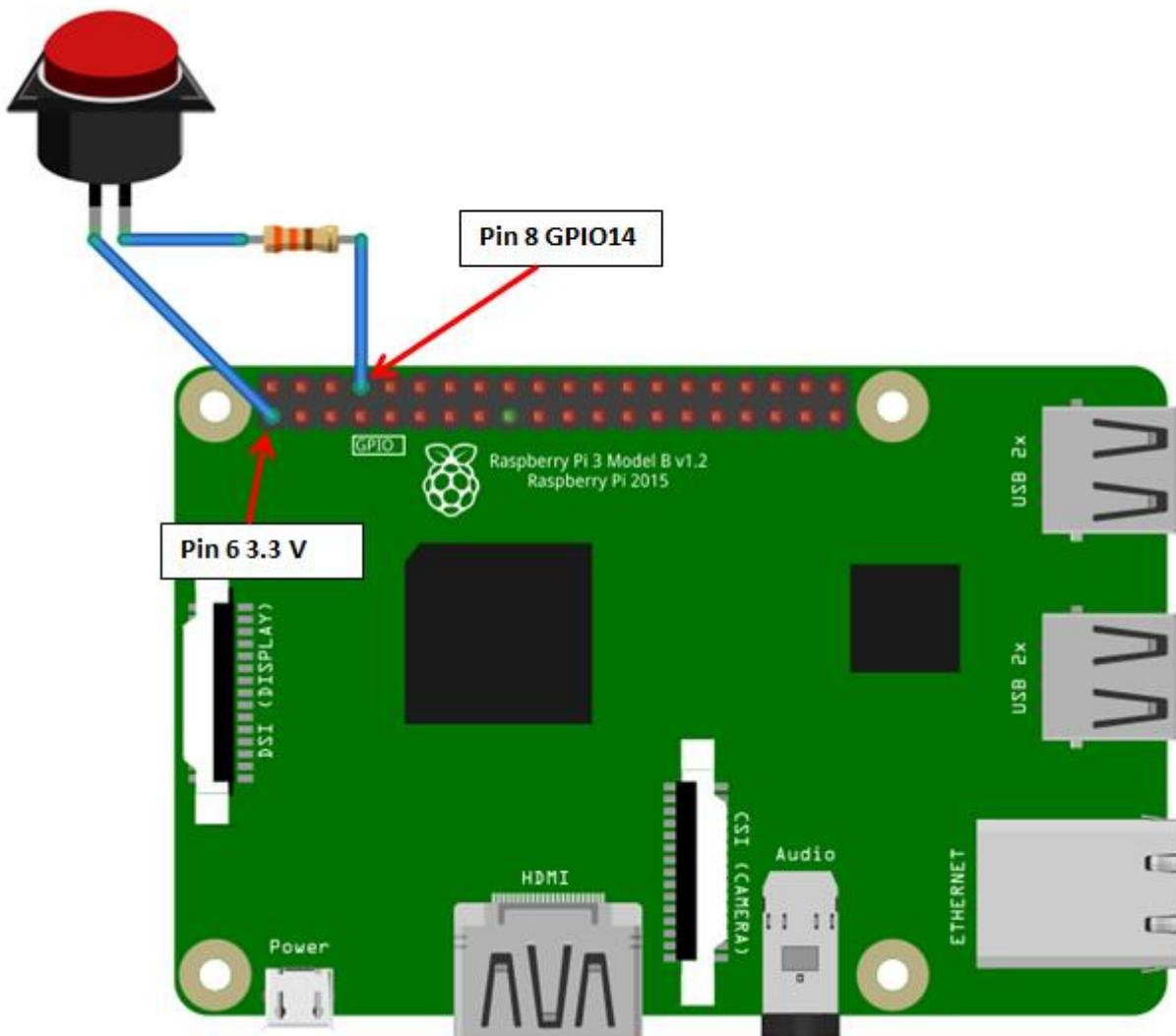
Schematic of Internal Resistor pulling the GPIO pin low\*
