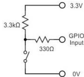
GPIO input is LOW (0) when switch is closed
