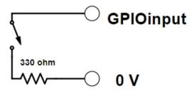
\* This configuration requires that you configure the internal pullup/pulldown resistors appropriately. Refer to the GPIO Inputs section for more detail.
