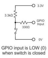
Graphical wiring of external Resistor pulling the GPIO 14 pin low.
