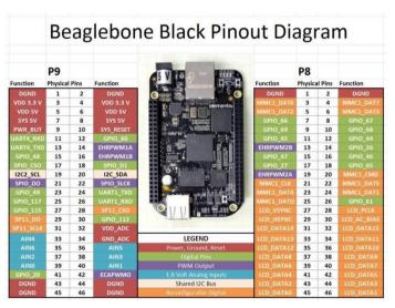
The GPIO pins are in a floating state and you will have to "force" it high (a positive voltage) or low (ground). This is done by connecting a resistor from the GPIO pin to either 3.3V (pulling high) or to ground (pulling low). This can be accomplished through a setting in the FPP GPIO Inputs page or by wiring a resistor in your circuit (it is not recommended to do both).
