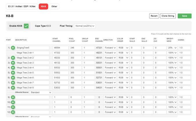
The capes from KulpLights.com can drive 800 pixels per port at 40 fps (roughly 1600 per port at 20 fps). Some controllers(like the KulpLights.com line of controllers)can also drive other components to control additional pixels like an Expansion Board, Differential Expansion Board, Differential Receiver, or Smart Differential Receivers.
