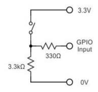
GPIO input is HIGH (1) when switch is closed
